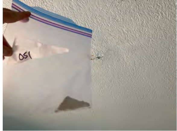
LTBA-006-PLM-051 Ceiling Texture (off-white) in Room 212.
